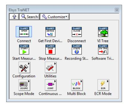
The upper part of the palette holds the most important functions, as connecting to the device and starting measurements. The two sub palettes "Configuration" and "Utilities" hold functions to configure the input settings and to have an easier access to certain hardware features. Finally at the bottom each of the four different recording modes has a sub palette on his own. Each sub palette contains a VI to configure the corresponding mode and VIs to read out the data recorded by this mode.
