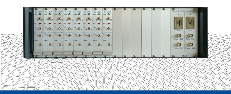
The device EL-BULT14 is able to produce TTL trigger pulses out of analog signals from optical (Laser), reluctance, capacitive and eddy-current sensors. The main application of the EL-BULT14 is to convert sensor signals to TTL pulses in structural health monitoring and vibration measurements of compressors and turbine blades.
