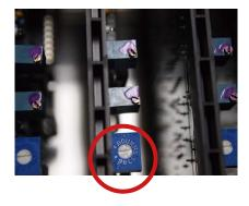
By installing the jumper J2, the hysteresis will be increased by a factor of approx. 3 (e.g 30 mV to 1.5 V at gain=1). This may be helpful at the use of reluctance sensors.
