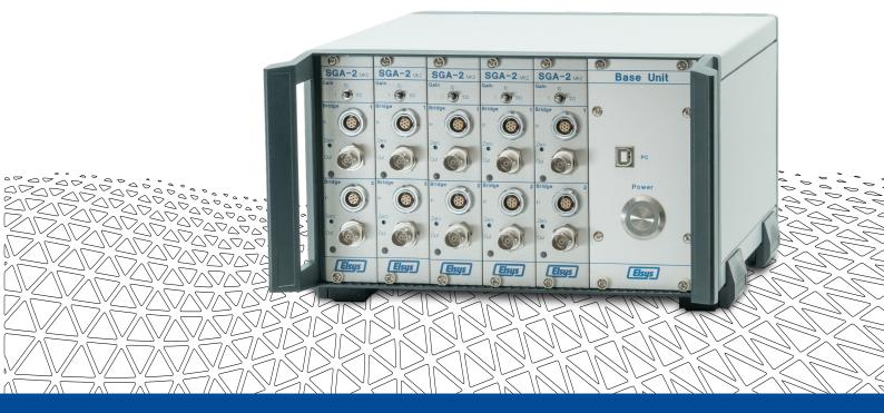
The SGA-2 strain gauge amplifier is designed as a differential frontend amplifier for connecting full, half or ¼ bridge strain gauges with internal bridge termination. The SGA-2 is designed for connection to a high-precision Elsys transient recorder, but is also suitable for any other data acquisition system.
