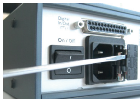
Changing the inlet protection fuse
